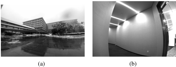
Fig. 2: Representative scenarios when perception system will fail by only using a LRF (a) or a camera (b). (a) In front of building on campus when all structures are far away, and (b) feature-less room in a building.
