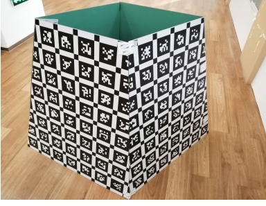
Fig. 3: Calibration ‘Pyramid’ for in-factory calibration, with April tags [23] on each surface to provide visual constraints and metric scale. Our design makes it easy for a robot to observe multiple surfaces simultaneously, to increase the total number of measurements. Note that each surface is not perpendicular to ground planes such that the roll and pitch of LRF is identifiable. This calibration pyramid is hollow so portable and of low cost.
